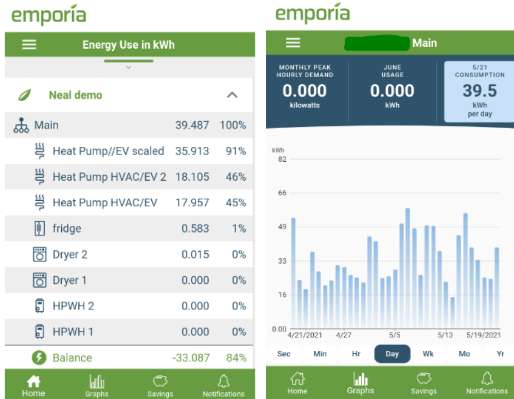
Figure 6. Example of a User Interface for a HEMS for Emporia Energy Device
